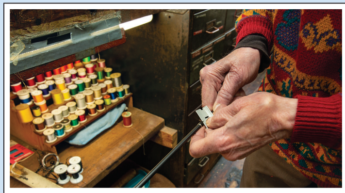
Replacing a fishing rod guide requires careful removal with a razor blade.
